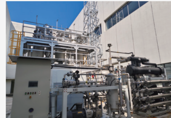
Dichloromethane Waste Gas Treatment System at the Lingang Industrial Park Site
